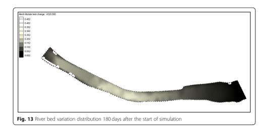
As shown in Figs. 12, 13 and 14, no variation was observed in the right bank of the upstream based on the results of simulation for longitudinal distance of approximately 1.1km from the upstream to downstream in analyzed section. The sedimentation of 0.15 m to 0.30 m occurred from the No. 3 to No. 6 sections which are the right banks of downstream. Later, the sedimentation of longitudinal section in downstream was found to decrease sharply.
