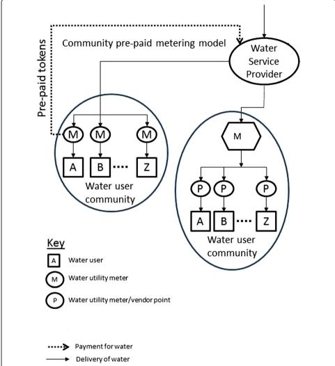
**Fig. 3** Conceptual Prepaid Metering Model. The communal prepaid meters are activated using tokens that are bought from the water service provider. The tokens are uploaded with credit at designated pay-points and water users can draw water up to the amount credited in the token. There were 91 communal prepaid meters installed in the network in Nakuru. The prepaid meters were installed to improve the quality of water service delivery to 15,000 people in the nine low-income settlements in Nakuru
